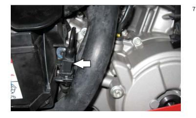
Locate and unplug the connector pair for the bike's Crank Position Sensor.
