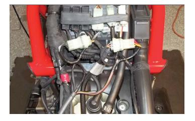
6 Attach the connectors from the PC6 to the stock wiring harness.
