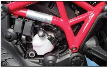
9 Locate and unplug the stock ignition coil connectors on the left side of the engine.
