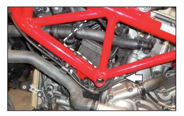
8 Unplug the stock Crank Position Sensor.
