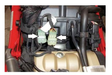
3 Unplug the 6 pin and 3 pin connectors on the back of the air box.
