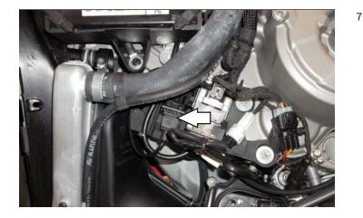
Locate Crank Position Sensor. Cut the zip tie holding the connector in place. Unplug the connector
